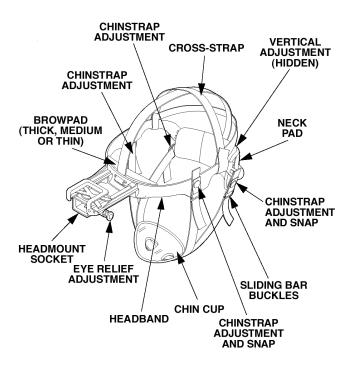
Figure 2-13. NVG Headmount Adjustments.
